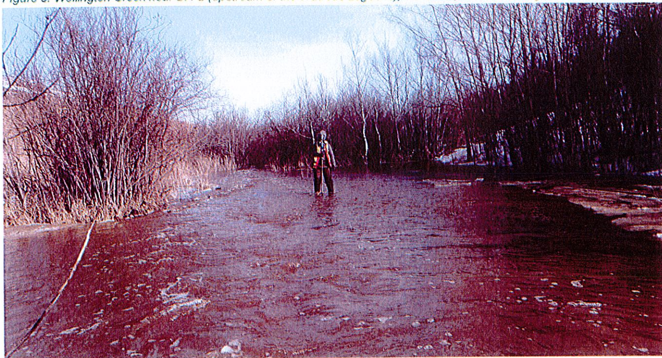
Figure 6: Freshwater Lake inflow near DA-3, March 15, 2015. Discharge is 1.60 \text{ m}^3/\text{s} .
